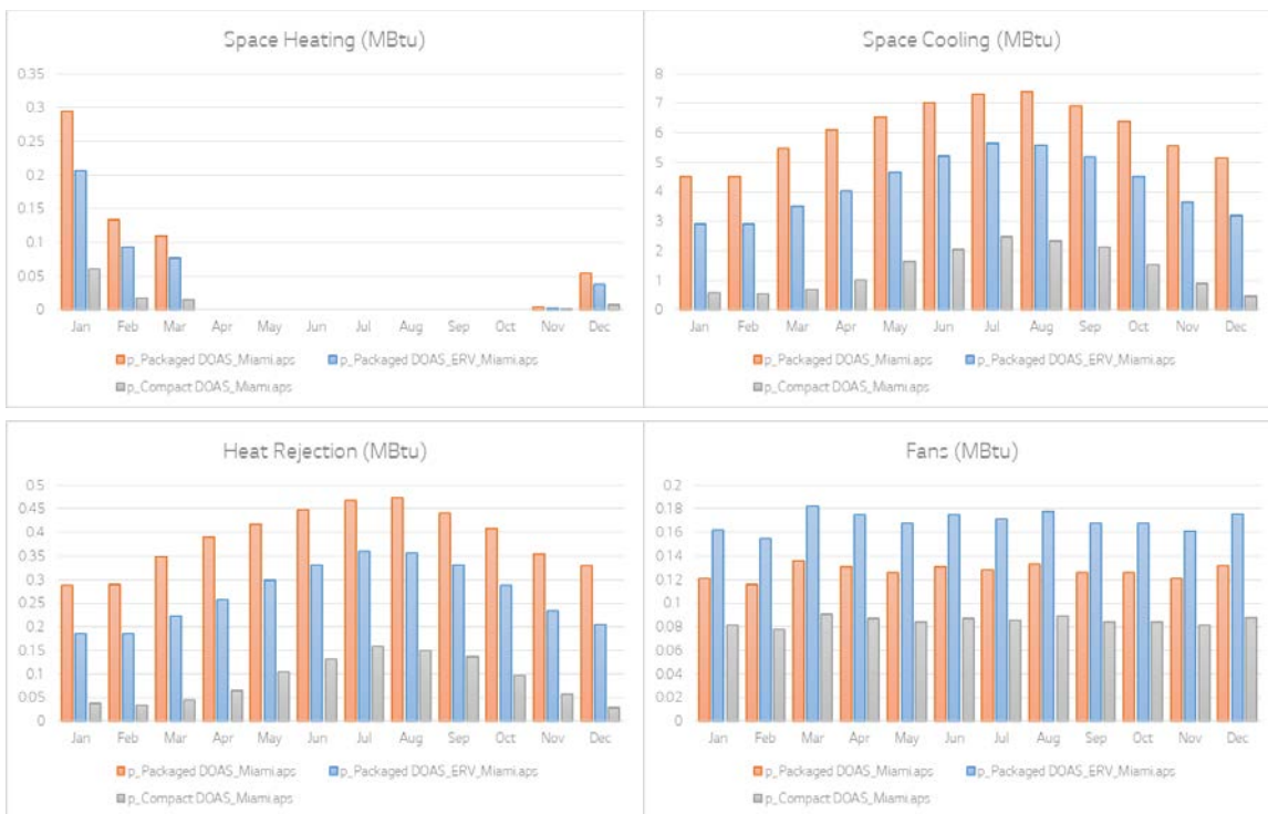
Figure 28: Ventilation Air Conditioning Energy (MBtu) - Miami.
