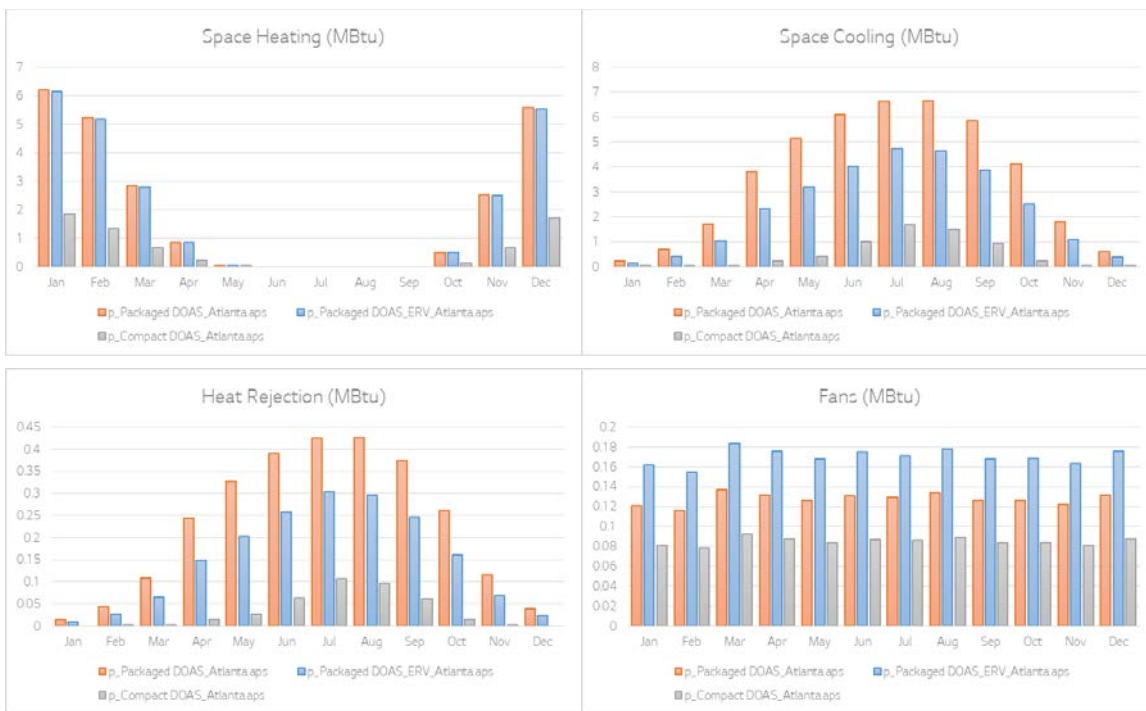
Figure 32: Ventilation Air Conditioning Energy (MBtu) - Atlanta.
