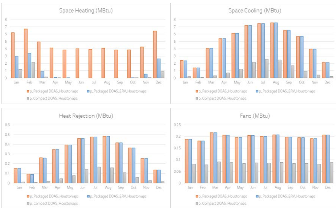
Figure 30: Ventilation Air Conditioning Energy (MBtu) - Houston.
