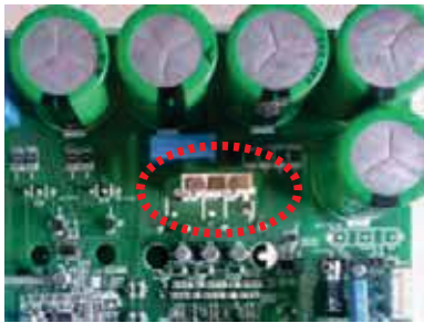
Figure 46: ARUN060GSS4 and ARUB060GSS4 Error No. 22 Compressor Terminal and Wiring Connections.
