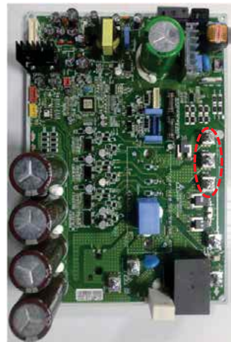
Figure 50: ARUN060GSS4 and ARUB060GSS4 Error No. 29 Compressor Terminal and Wiring Connections.
