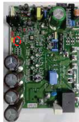
Correct Inverter EEPROM Installation Direction.
