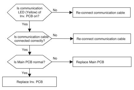
\* The method of checking Main PCB and Inv. PCB (If normal, communication LED blinks)
