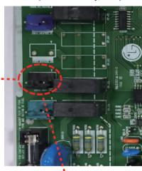
\*\* Confirm the 4way valve coil is inserted to the end
