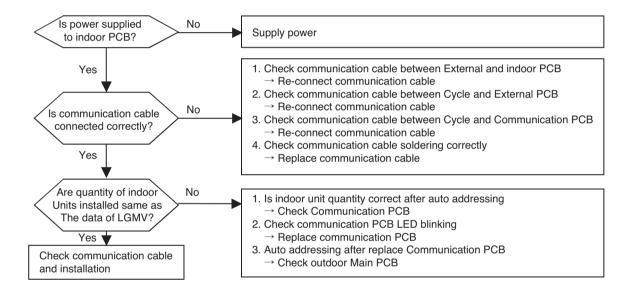
In case of CH53, almost happened with CH05, the indoor units not operated actually are normal so check with same method of CH05. and additionally check as shown as below and above flow chart
