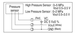
The pressure sensor is composed like the circuit picture shown above. If DC 5 V voltage flows on red and black wire, voltage would be made between the white and black wire. The pressure which is equivalent to the pressure output is shown in the table above.
