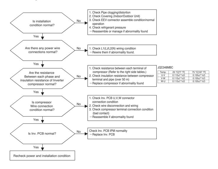
\* Measuring resistance between each terminal of compressor
