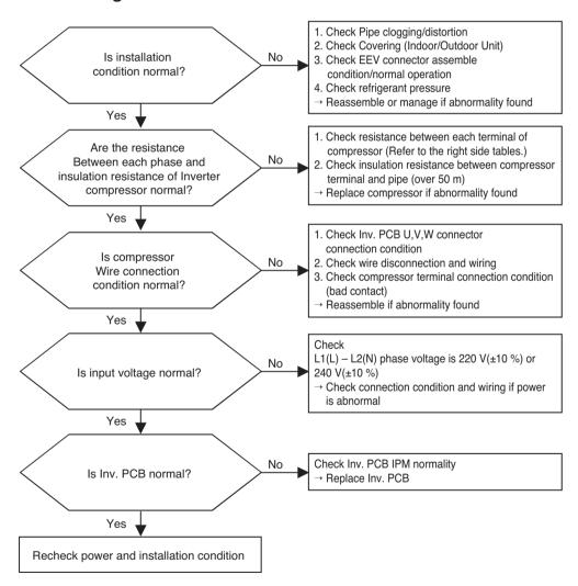
\* Measuring resistance between each terminal of compressor
