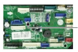
Float switch Housing (CN-FLOAT)
