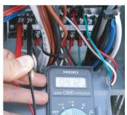
\* If the DC voltage between communication terminal A, B of indoor unit is fluctuate within (-9 V~+9 V) then communication from outdoor unit is normal
