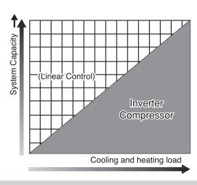
Inverter linear control as cooling and heating load increasing
