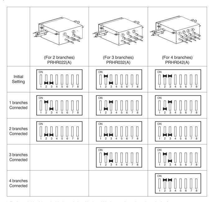
★ Each model is shipped with the switches No.2 and No.3 pre-adjusted as above in the factory.
