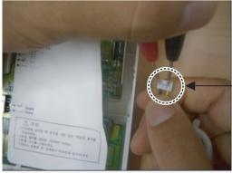
Checking communication cable connection status
