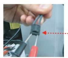
Location of 4way valve connector on Main PCB(marked as 4way,CN09)
