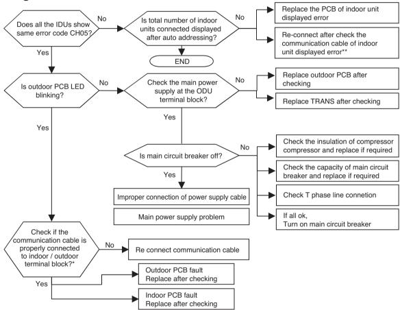
\* (Note1) communication from IDU is normal if voltage fluctuation(-9 V ~ +9 V) exists when checking DC voltage of communication terminal between IDU and ODU
