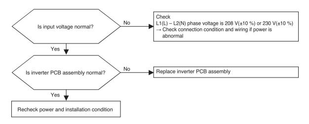
\* Measuring input voltage
