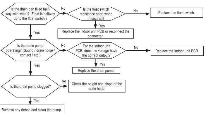
\* If the float rises higher than half its height, then the circuit opens and the unit automatically stops.
