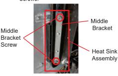
Figure 69: Detachingthe IGBT Screws.
