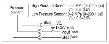
See the pressure sensor schematic at left. DC 5V will to be measured between red and black wires. DC voltage measured between white and Black wire corresponds to charts above.
