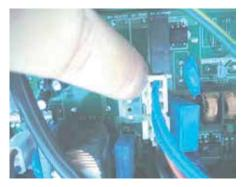
\*\* Indoor PCB Drain Pump Connector (Check Electrical Input; Marked as CN-DPUMP
