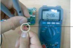
Measure the resistance of outlet pipe temperature
