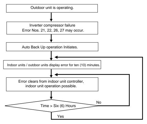
Example: Slave1 Outdoor Unit Inverter Compressor 1 fails (Error No. 21 displays)
