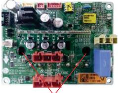
Check fan connection installation.
