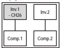
If Inverter 2 has CH26 displayed, then Comp. 1 is defective.
