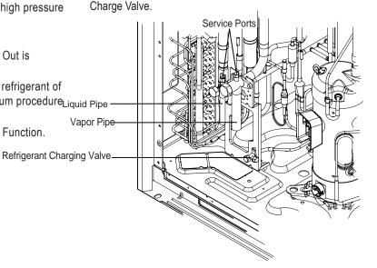
Figure 28: Close Up of Heat Recovery Service Ports and Refrigerant
