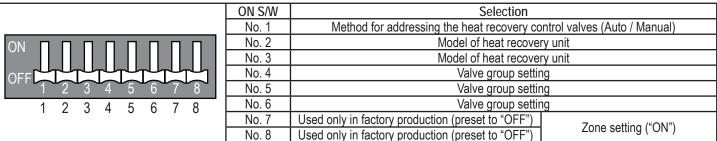
Selecting the Heat Recovery Unit Valve Addressing Method (Pipe Detection) (Auto / Manual).
