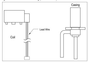
Figure 54: Removing and Assembling the Coil.
