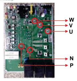
Table 65: Checking the Inverter IGBT / IPM.
