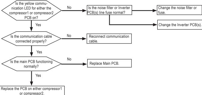
Checking the Main PCB and Inverter Compressor 1 / Inverter Compressor 2 PCB (If operating normally, the communication LED will blink)
