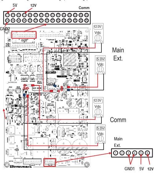
Figure 82: Multi-Meter (Note the Probe Color).
