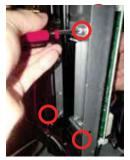
Figure 70: Removing the Inverter PCB.
