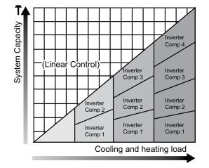
Inverter linear control as cooling and heating load increases
