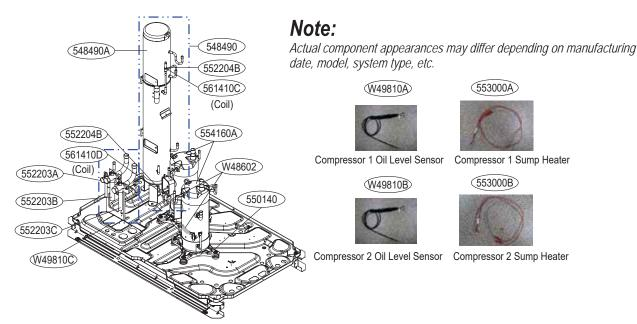
Table 100: Temperature Sensor Parts List for 8- and 10-Ton (Large Frame) Outdoor Units.
