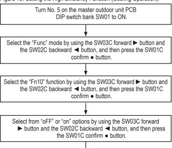
Press the SW01D Reset Button one (1) time to reset PCB. The High Efficiency Function in Cooling Operation is set.
