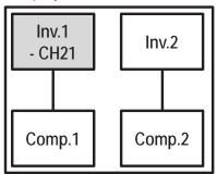
If Inverter 2 has CH21 displayed, then Comp. 1 is defective.
