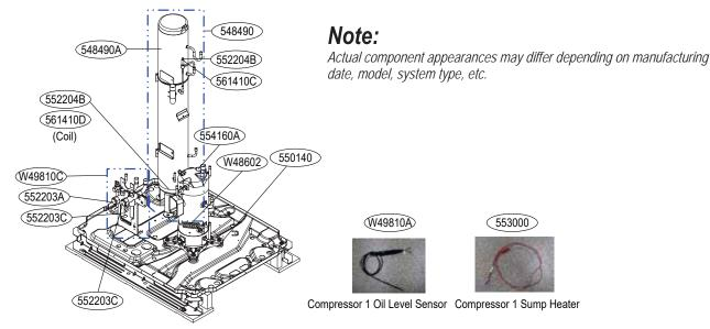
Table 98: Temperature Sensor Parts List for 6-Ton (Small Frame) Outdoor Units.
