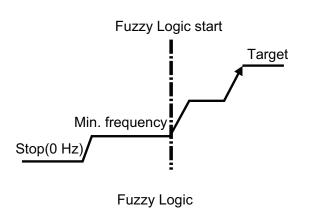
Figure 2: Inverter Linear Control Chart.
