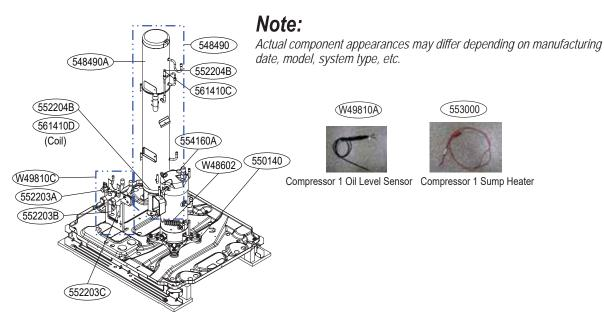
Table 99: Temperature Sensor Parts List for 8- and 10-Ton (Large Frame) Outdoor Units.
