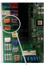
Confirm the four-way valve coil is completely inserted.
