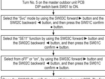
Press the SW01D Reset Button one (1) time to reset PCB. The Fan Low Sound in Heating is set.
