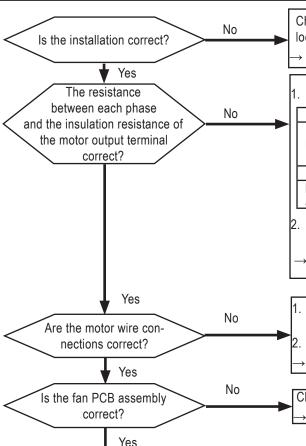
Check if the outdoor unit fan motor assembly is correct or if it is locking up.
