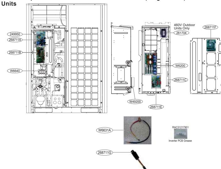
Table 96: PCBs - Internal View for 8- and 10-Ton (Large Frame) Outdoor Units Harness List.
