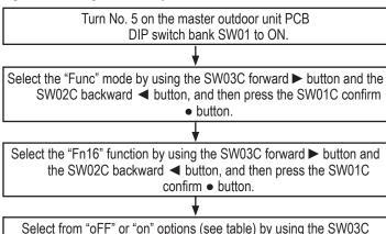
forward ▶ button and the SW02C backward ◀ button, and then press the SW01C confirm • button.
