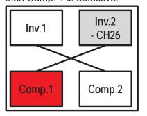
If Inverter 1 consistently displays CH26, then Inverter 1 is defective.
