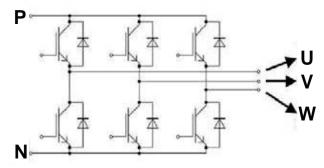
Figure 58: Location of IGBT / IPM Terminals (Appearances Will Vary Depending on Model).
