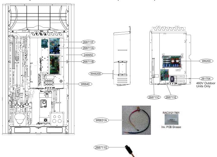
Table 95: PCBs - Internal View for 6-Ton (Small Frame) Outdoor Units Harness List.
