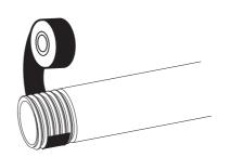
2 Attach the discharge pipe to outlet of the T&P relief valve. The discharge pipe must pitch downward from the valve to allow complete drainage of both T&P relief valve and discharge pipe.
