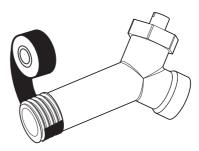
**2** Install the drain valve in the opening marked "Drain Valve".
