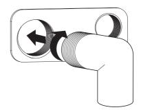
**3** Using an approved sealant, insert the PVC pipe into the female end. Condensate drain must be piped to an adequate drain.
