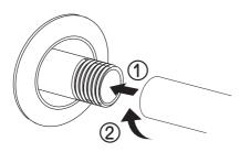
For ease of disconnecting the water heater for service or replacement, the installation of unions is recommended on the water connections.
