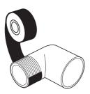
**2** Attach elbow with 3/4" slip &3/4"NPT to the primary drain connection.
