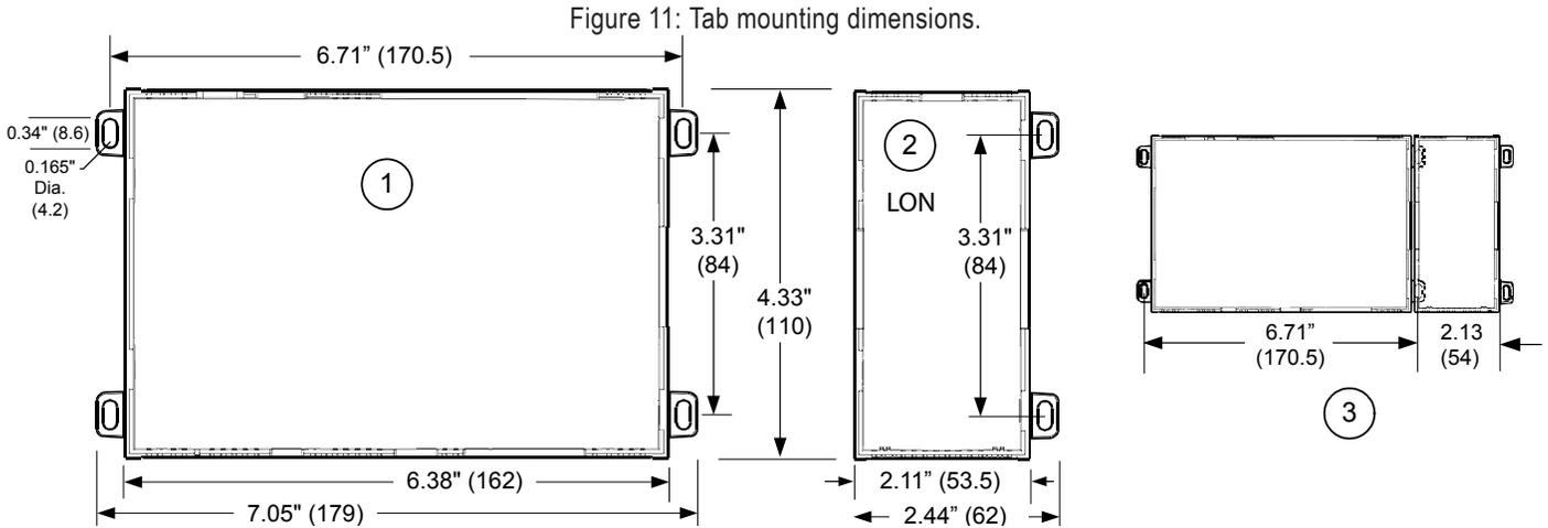
**1** = MultiSITE VM3 controller. With no optional LON modules added, allow at least 1.5" (38mm) clearance around all sides, and minimum 3" (76mm) at bottom for WiFi antenna.
