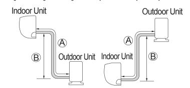
Figure 44: Single Zone High Efficiency Wall Mount System Layout.
