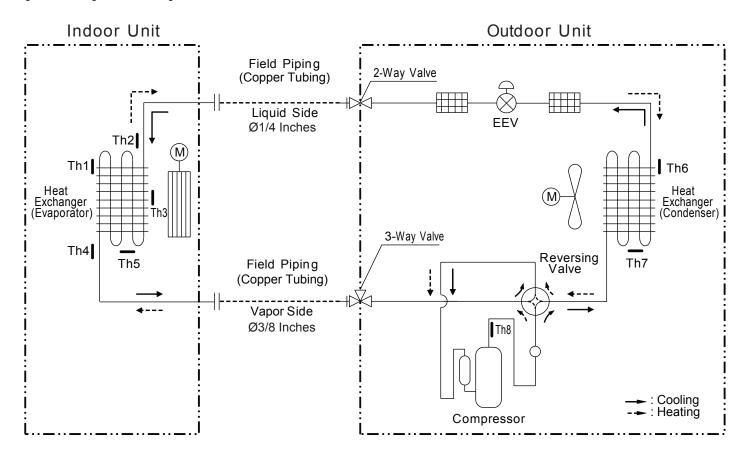
Table 8: Single Zone High Efficiency LSN/LSU090-120HSV5 Thermistor Details.
