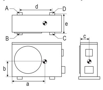
Table 5: LSU090-120-181HSV5 Outdoor Unit Corner Weight and Center of Gravity Dimensions.
