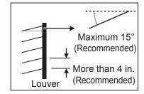
Figure 41: Using "S" Type Louvers.
