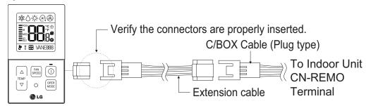
Figure 27: Wired Controller Connection on the Indoor Unit Terminal Block.
