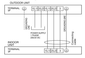
Figure 25: LS181HSV5 System Electrical Connections.
